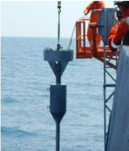
LARS operations (lifting the piston into the cradle).
