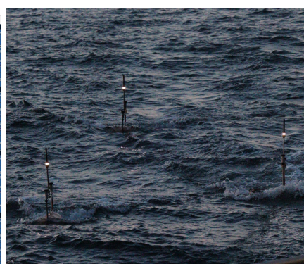
Geo-POS antennas mounted on source, head and tail streamer for a single-channel survey - blinking codes report the situation of each buoy apart from the software interface.
