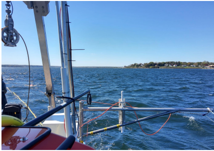
An at least 4 m long outrigger remains one of the most important requirements to deploy the streamer out of the turbulence of the prop wash (left: small vessel; right: large vessel operations).
