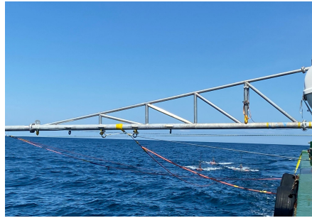
An at least 4 m long outrigger remains one of the most important requirements to deploy the streamer out of the turbulence of the prop wash (left: small vessel; right: large vessel operations).
